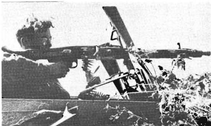
TOP LEFT: The basic infantry MG34 model. With its butt and bipod removed this gun was fitted into AFV mountings.
