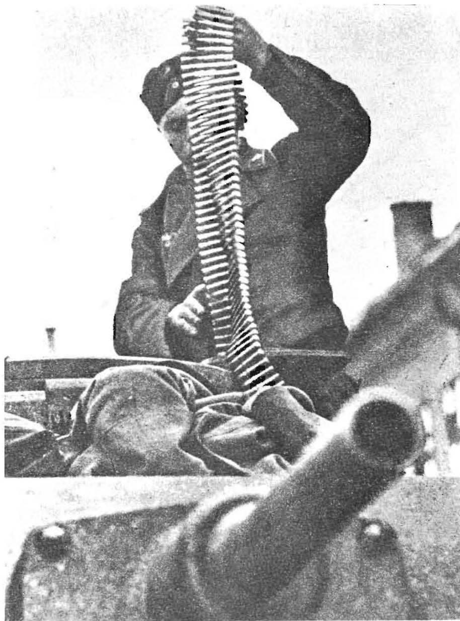
7.92 mm machine gun belts being loaded into a Pzkw III. These 100 round belts for the co-axial and bow MG34's were loaded into canvas bags when stowed inside the vehicle.
