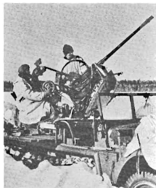
2 cm Flak 38 mounted on a Sdkfz 10 'Demag' 1 ton half-track.
