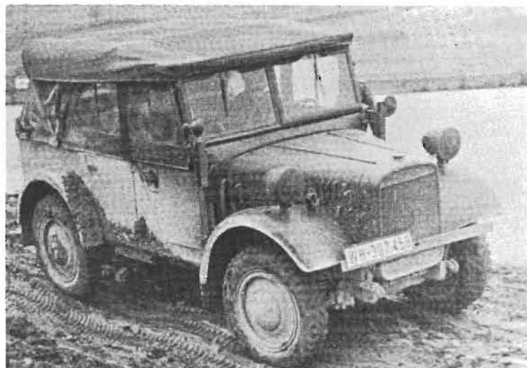
ABOVE: Sdkfz 2 Stöwer 40 light car of the Wehrmacht. This type of body-work was standardised to fit on the commercial light car chassis that were available.
