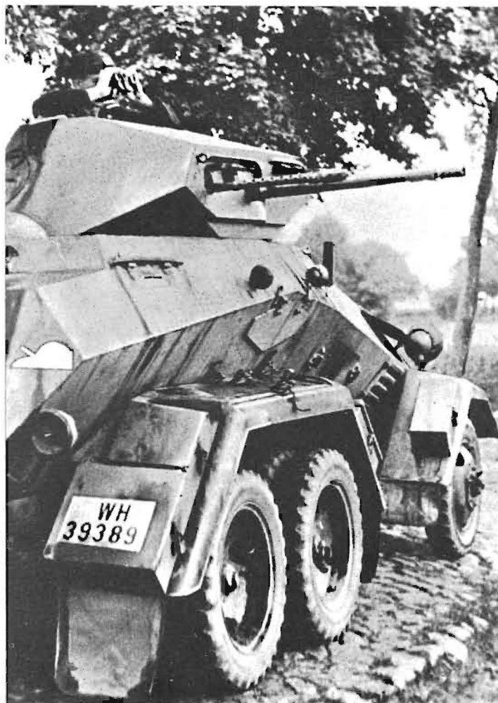
BELOW: The smallest German AFV gun, the 2 cm KWK here mounted in a Pzspw (6 rad) Sdkfz 231 heavy armoured car.
